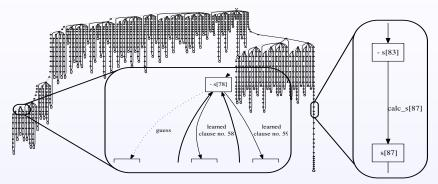
Figure: Graphviz visualisation of an example search for the Crypto-1 cipher's states. The tree is read from left to right, top to bottom: the left- and bottommost pentagon is the first conflict clause, the right- and bottommost circle is the satisfying assignment.
